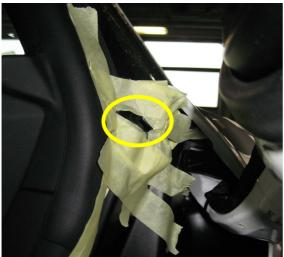
6. Apply the 3M sealant as shown in the picture, with particularly care to not soil the bodywork.
